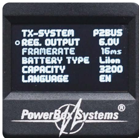
Basics screen, where language, battery type and capacity, output voltage and servo frame rate are set
