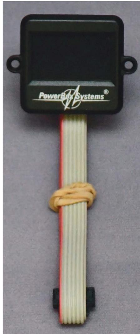
OLED display supplied in the Mercury package
