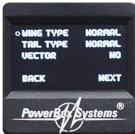
Setup Assistant initial screen, where wing type, tail type and any vector operation is set
